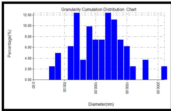
Fig. 5-d. Bar chart of particle size distribution of silica micro particles.
