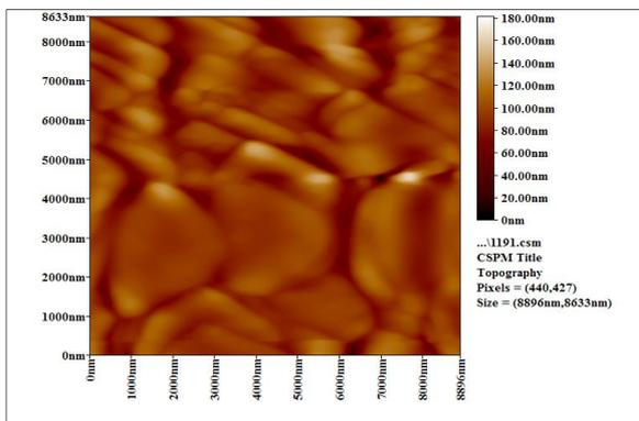
Fig. 5-d1. AFM for SiO<sub>2</sub>micro particles with average diameter of (1017.96) nm.
