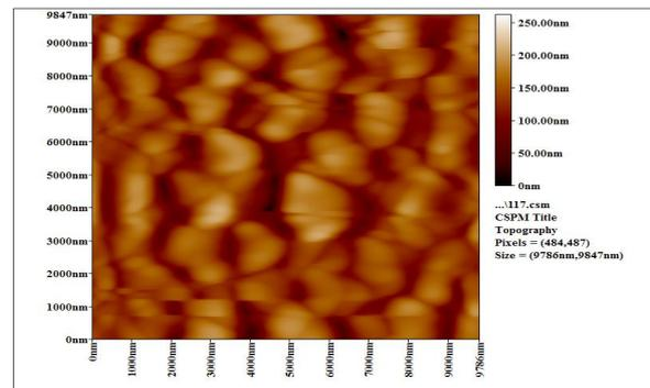
Fig. 5-c1. AFM for ZnO micro particles with average diameter of (896.81) nm.
