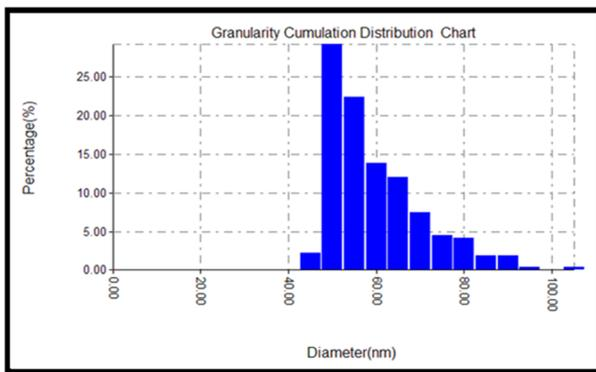
Fig. 5-a. Bar chart of particle size distribution of ZnO nanoparticles.
