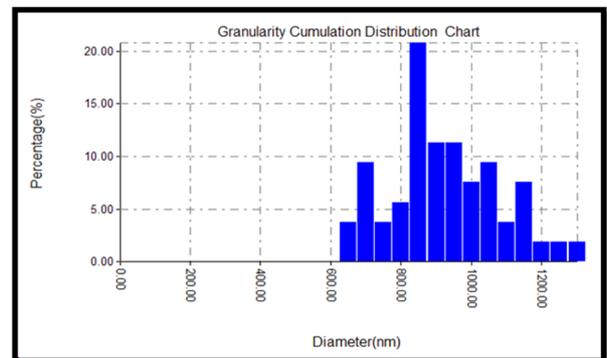
Fig. 5-c. Bar chart of particle size distribution of ZnO micro particles.
