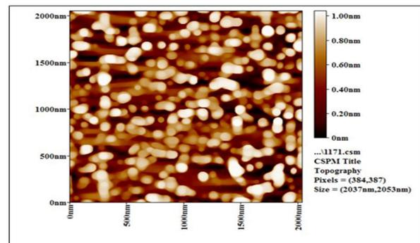
Fig. 5-b1. AFM for SiO<sub>2</sub>Nano particles with average diameter of (69.74) nm.
