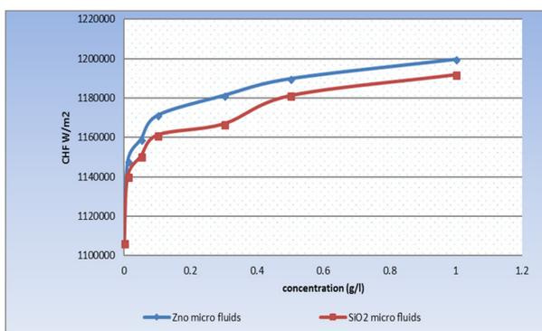
**Fig. 4.** CHF results for (ZnO, SiO<sub>2</sub>) micro fluid.
