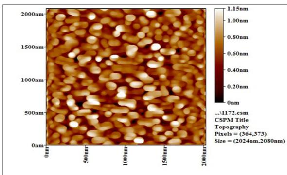
Fig. 5-a1. AFM for ZnO Nano particles with average diameter of (57.01) nm.
