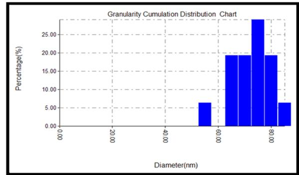
Fig. 5-b. Bar chart of particle size distribution of silica nanoparticles.
