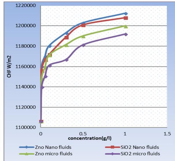
Fig. 6. comparison of CHF between (ZnO, SiO<sub>2</sub>) Nano and micro-fluid.
