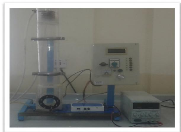
**Fig. 1. Photograph of pool boiling system with Ni-Cr wire heater for CHF measurement.**
