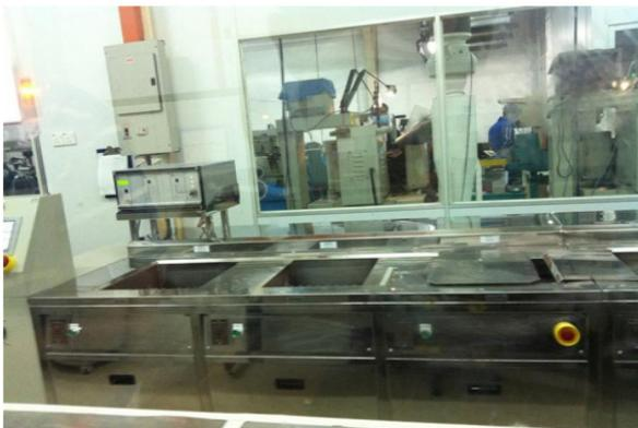
**Fig. 3.** The cutting insert was cleaned by ultrasonic with a detergent bath for different mixed detergent and time.
