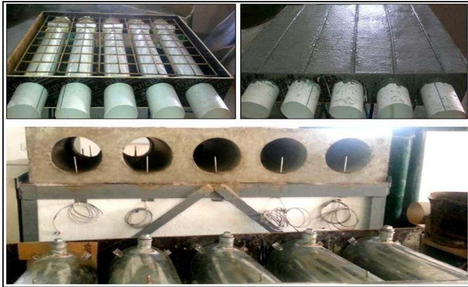
Fig. 4. Steps of manufacturing the ThermoDeck system
