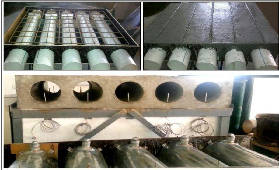
Fig. 4. Steps of manufacturing the ThermoDeck system
