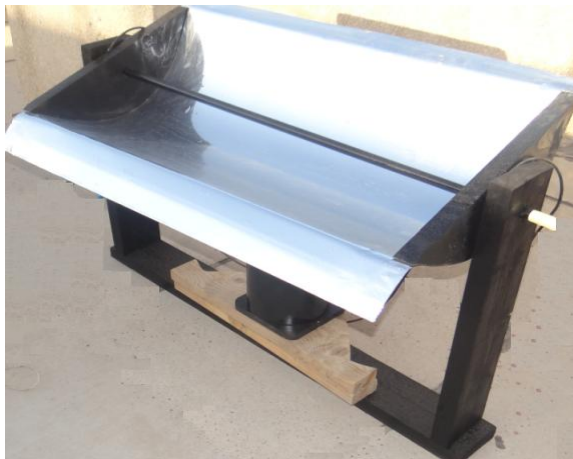
Fig. 4. The parabolic trough with reflective material and support frame.
