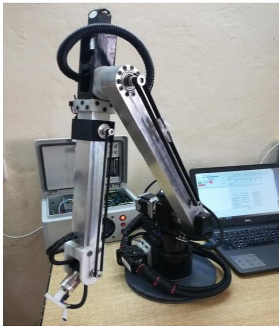
Fig. 1. Three Links Robot Manipulator 6 DOF.
