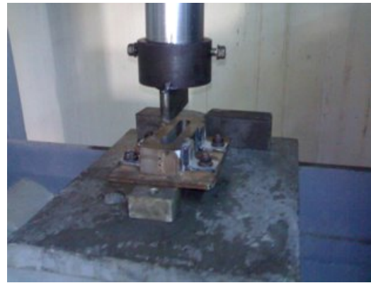
Fig.1. The Punch and Die Used in Squeeze Casting.
