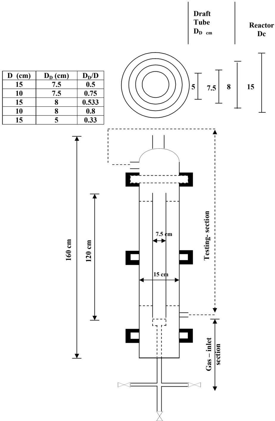
Fig. 3. Airlift Loop Reactor.
