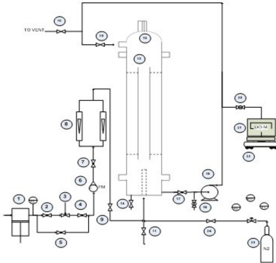
Fig.1. Experimental-Apparatus (1: Air Compressor; 2,4,5,7,17: Globe Valves; 3: Needle Valve; 6: Gas Meter; 8: Gas Rotameter; 9: Two-Way Valve; 10: Gas Distributor; 11,14,15,16,24: Gate Valves; 12: Draught Tube; 13: Column; 18,20: Ball Valves; 19: Centrifugal Pump; 21: Dissolved Oxygen Meter (Do-m); 22: Move Table; 23: Nitrogen Cylinder; PG, PCV: Pressure Control Valve Pressure Gauge).
