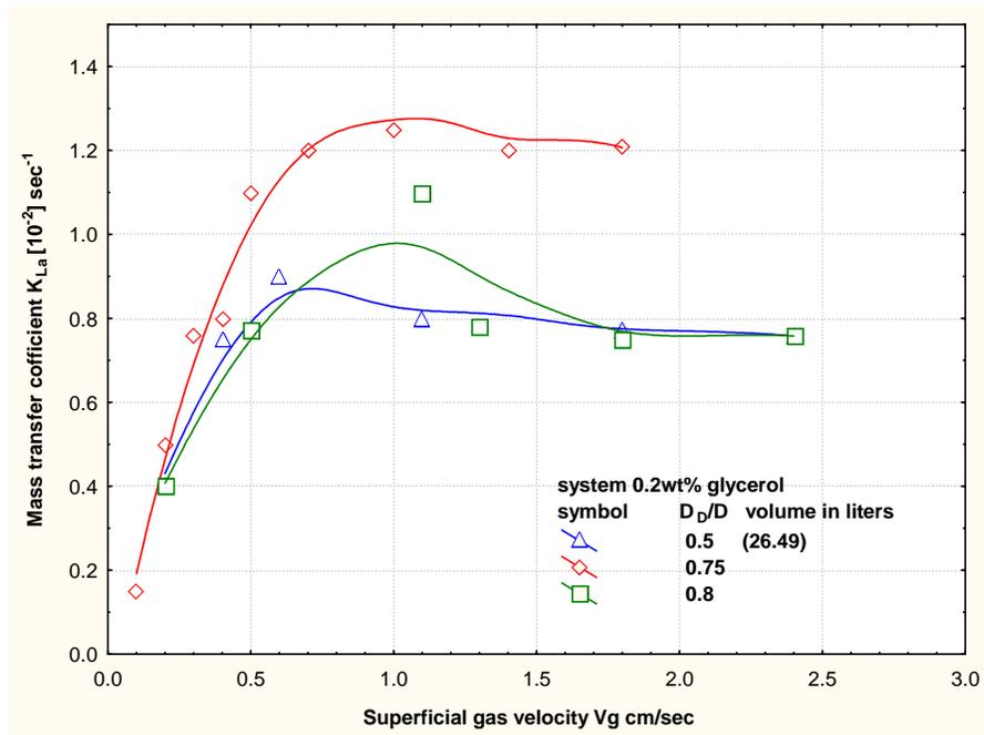
Fig.5. Influence of Draft Tube Diameter on Mass Transfer In Viscous Liquid Phase (Aqueous Glycerol).
