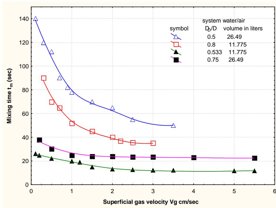
Fig.6. Effect of Gas Through Put and Draft Tube Geometry on Mixing Time in Airlift Loop Reactors of Different Sizes.
