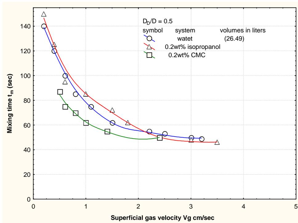
Fig.9. Mixing Times in Different Liquids as a Functions of Super Ficial gas Velocity.
