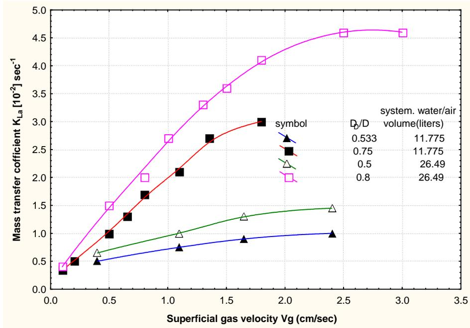
Fig.4. Effect of Gas Velocity and Draft Tube Geometry on the Volumetric Mass Transfer Coefficient in Airlift Loop Reactors of Different Sizes.
