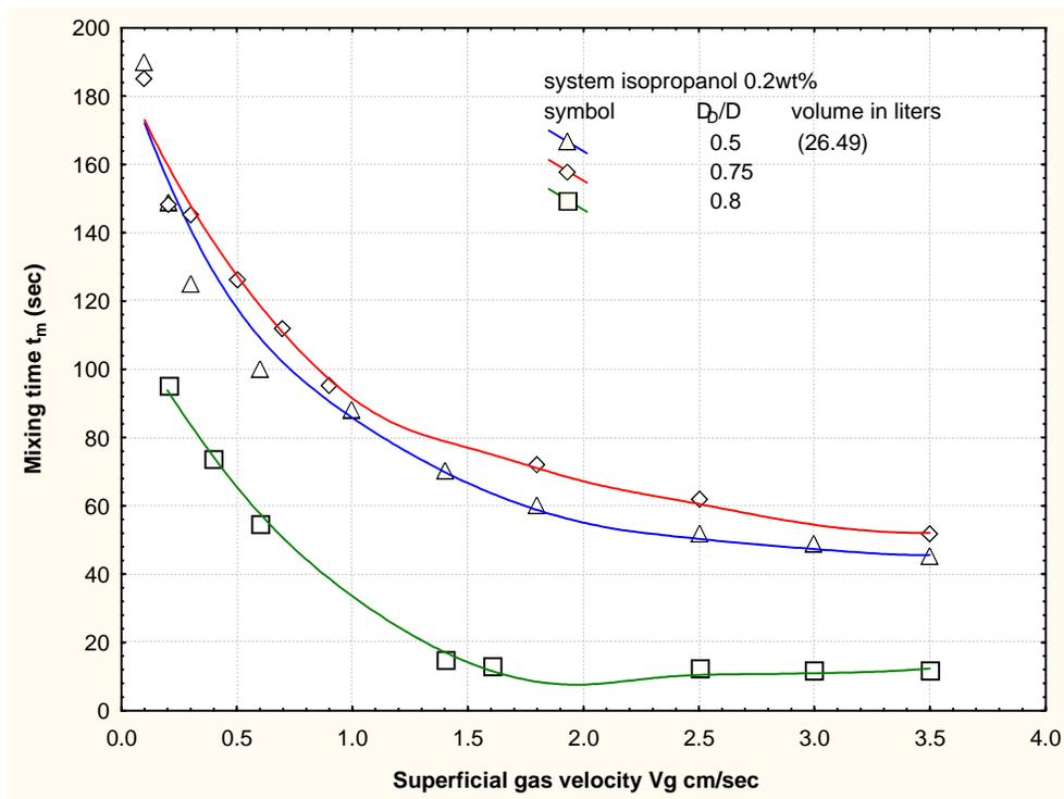
Fig.7. Mixing Time in Aqueous Solution of Isopropanol.
