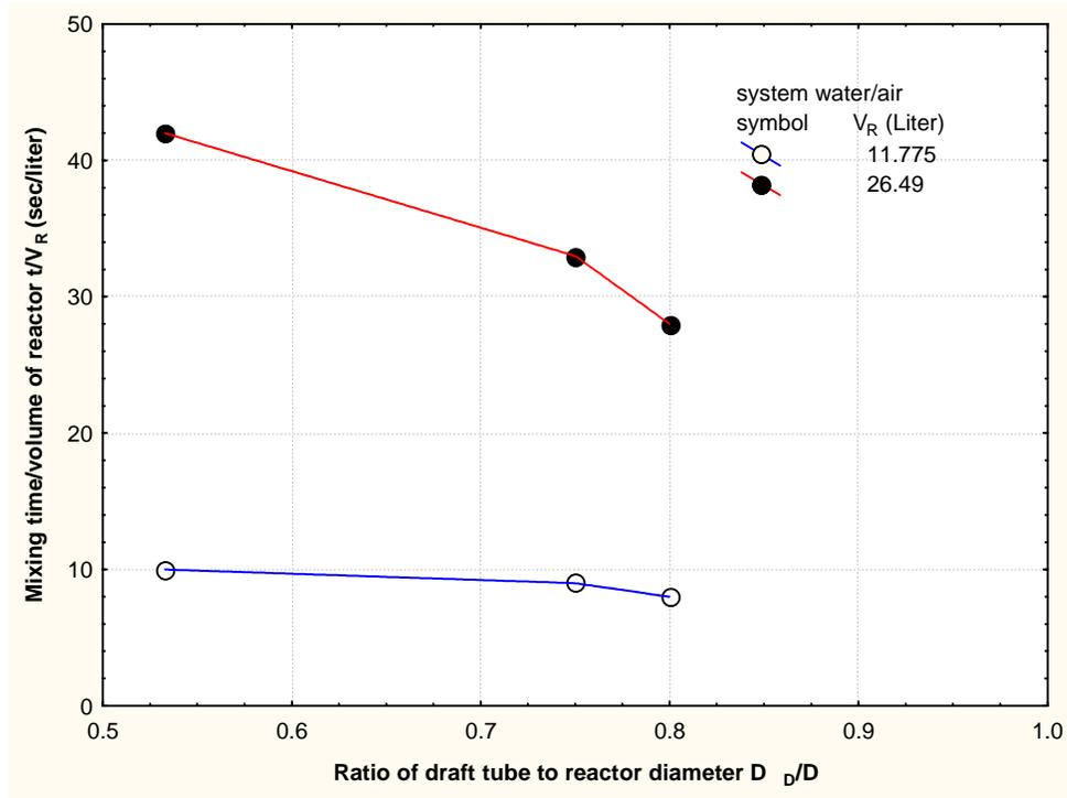
Fig.8. Mixing Time Per Unit Volume as a Function of Draft Tube to Reactor Diameter Ratio.
