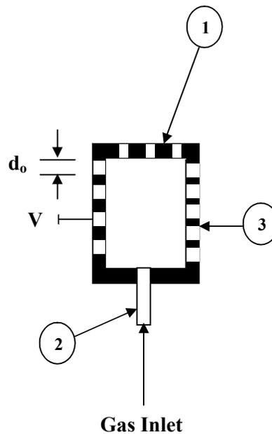
Fig.2. Gas-Distributor (1: Ceramic Material; 2: Pipe; 3: Hole).
