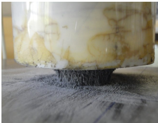
Fig.2. Magnetic Brush Formed between the Electromagnet Pole (North) and the Ferromagnetic Workpiece (South).
