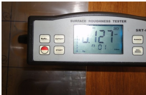
Fig.4. Measuring the Value of Ra Using Surface Roughness Tester (SRT-6210).
