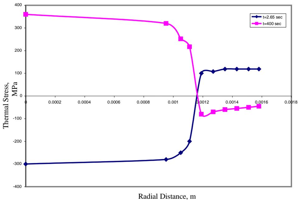
**Fig.9. Thermal Stress Distribution During and After Laser Spot Welding**
