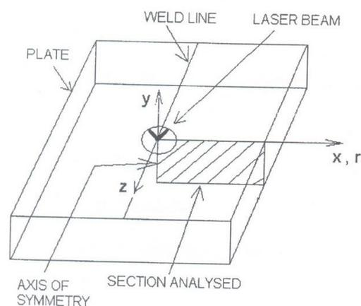
Fig. 1. Transverse Section of Thermal Model [13]
