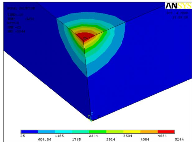
Fig.7. Temperature Distribution During Laser Spot Welding
