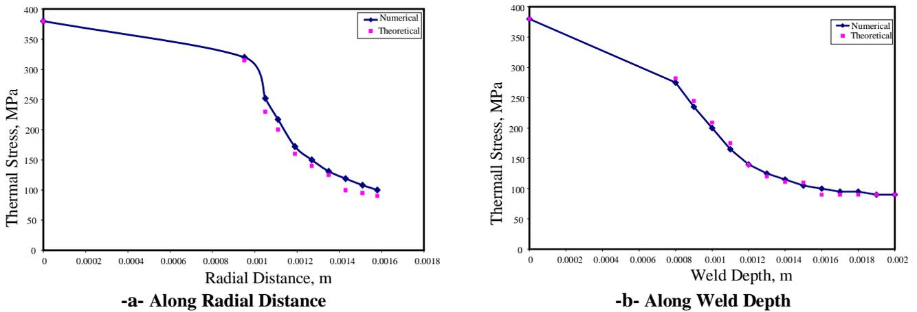
**Fig.8. Von Mises Thermal Stress Distribution After Laser Spot Welding**
