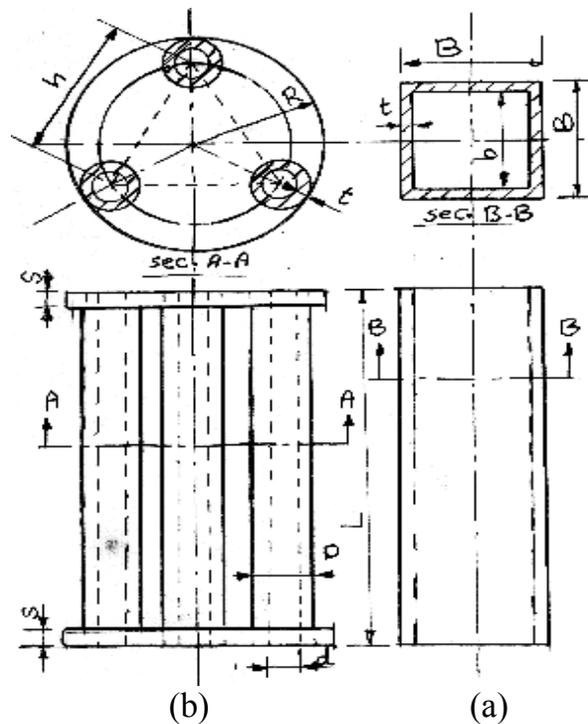
Fig.(2) (a) uni-tube configuration
