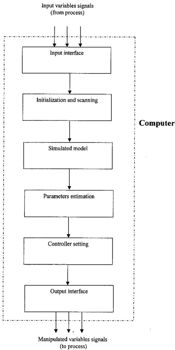
Fig.4. Block Diagram of the Computer Control Function.
