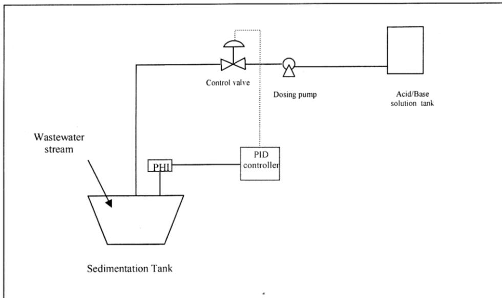
Fig. 2. Flow Diagram of PID Control System.
