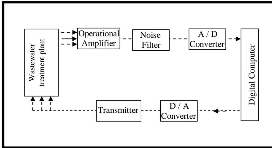
Fig. 3. Hardware Components of On-Line Control System.
