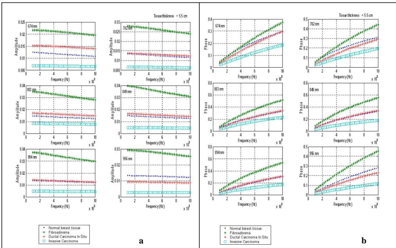
Fig. 8. a) The Amplitude (AC) of the Detected Laser Signal vs. The Modulation Frequency, b) The Phase Shift  $\phi$  of the Detected Signal vs. The Frequency for Laser Wavelength ( $\lambda = 674, 782, 803, 849, 894,$  and  $956$  nm) at Tissue Thickness  $5.5$  cm for Postmenopausal Female.
