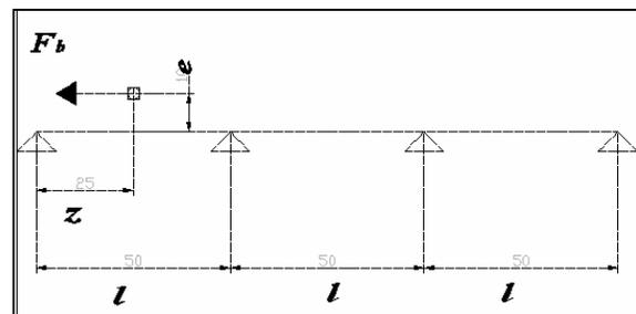
Fig. 2. Location of the Braking Force  $F_b$
