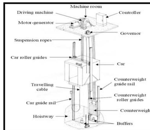
Fig. 1. Components of Elevators
