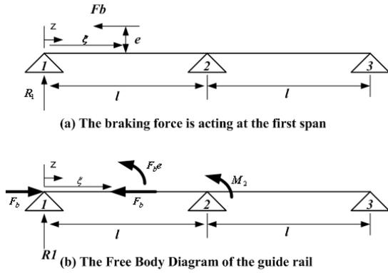
Fig. 5. F.B.D. of Guide Rail (at Field I)
