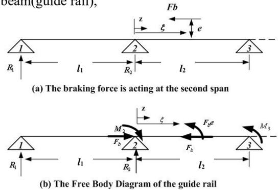
Fig. 6. F.B.D. of Guide Rail (at Field II)
