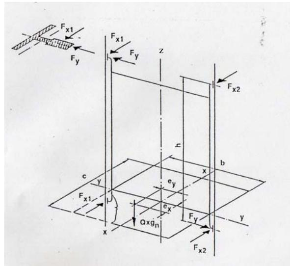
Fig. 7. Forces on guide rails during normal operation
