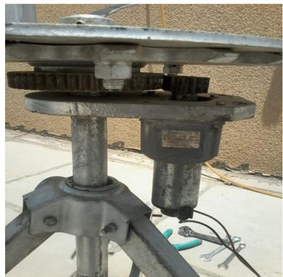
Fig. 2a. DC gear box (axial motion).
