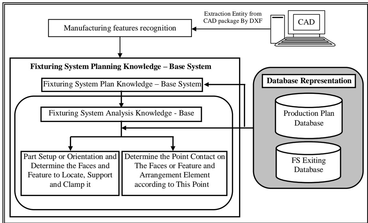
Fig.1. The (AFSP) System Architecture.
