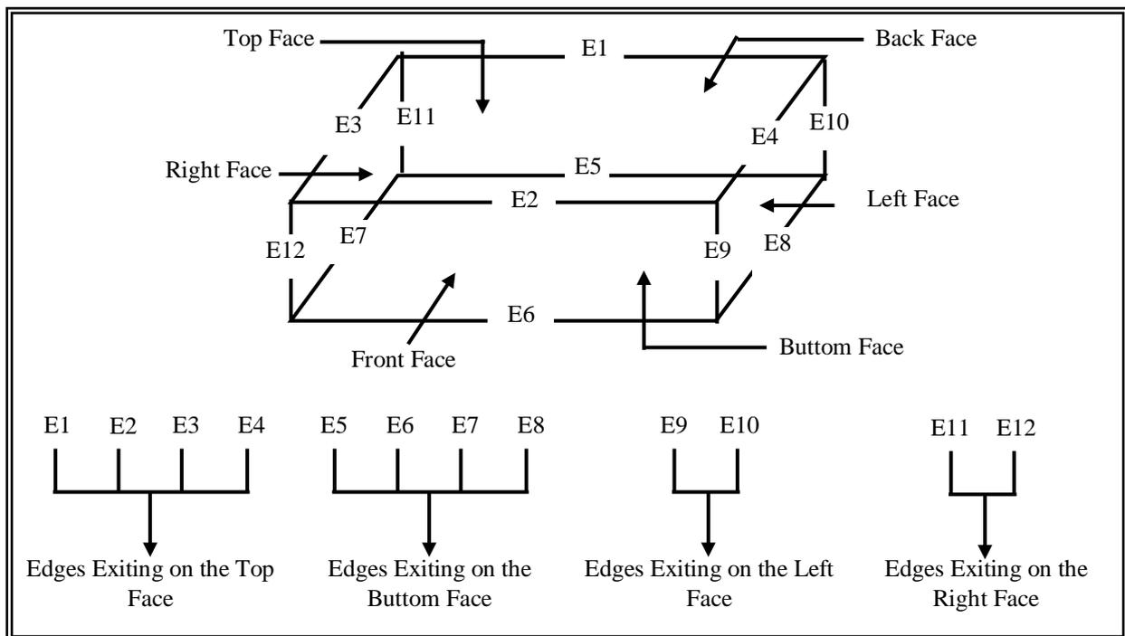
Fig.4. Relational Location of Machined Feature for Uniform Polyhedra Workpiece.
