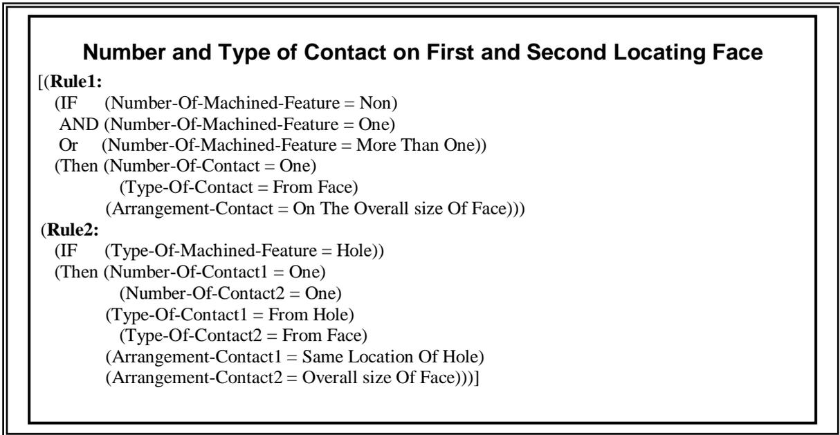
**Fig. 8. Examples of Rules Used For Determining Fixturing Planning.**
