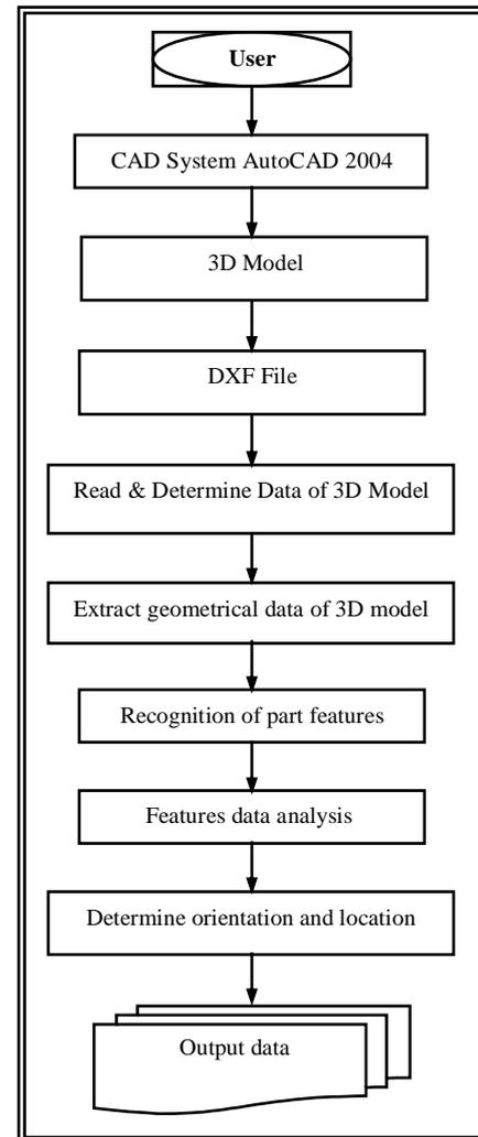
Fig.2. Algorithm for Recognition Features.
