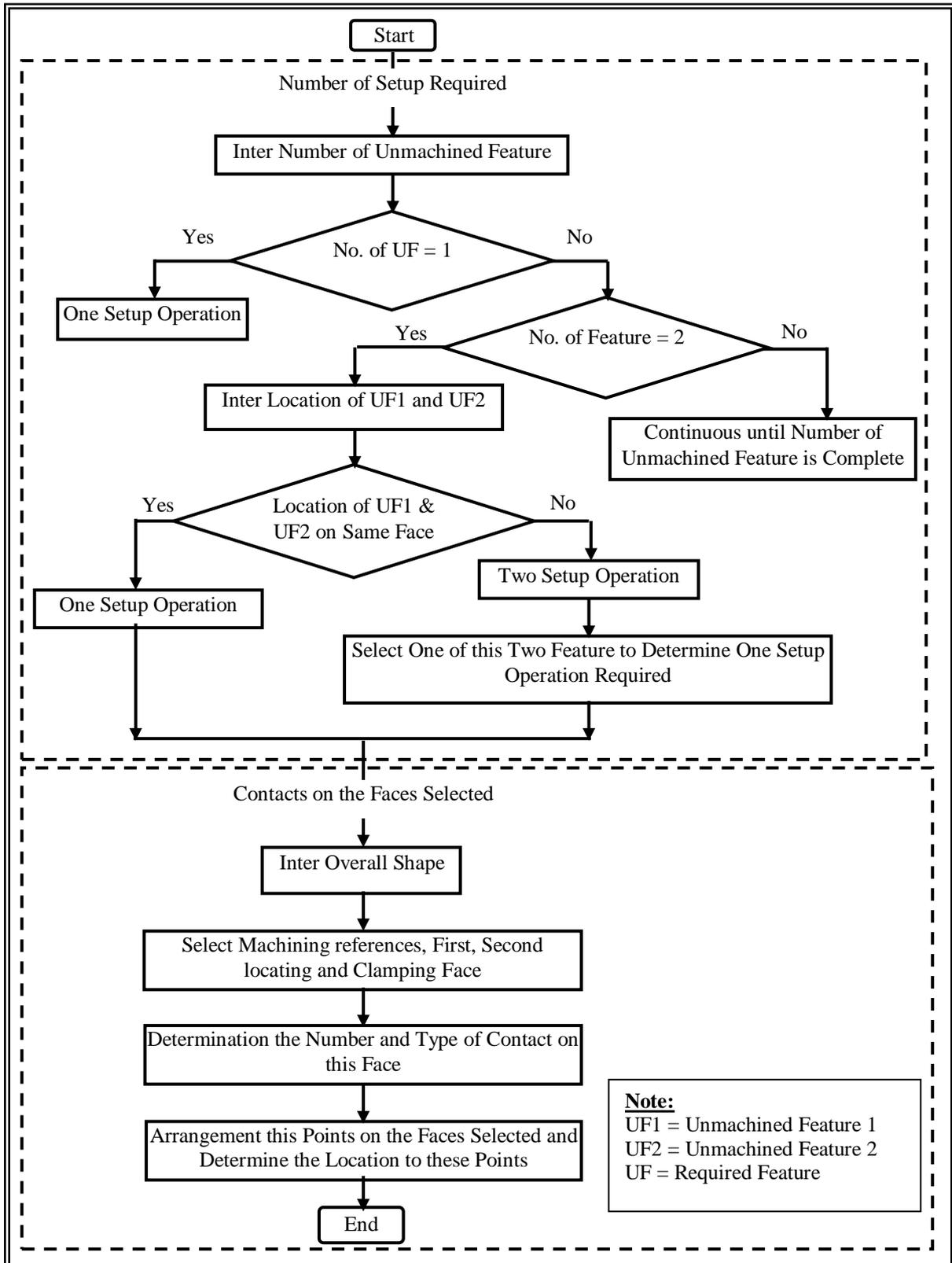
Fig.7. Flowchart for Fixturing Analysis.
