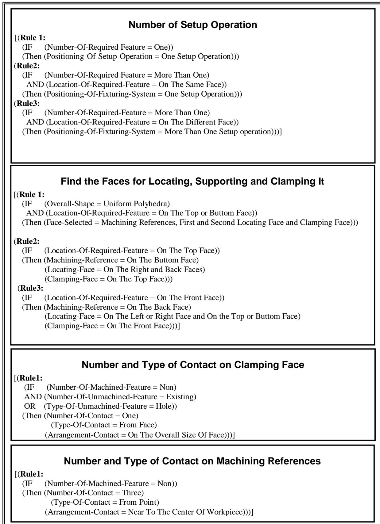
**Fig. 8. Example of Rules Used For Fixturing Planning.**
