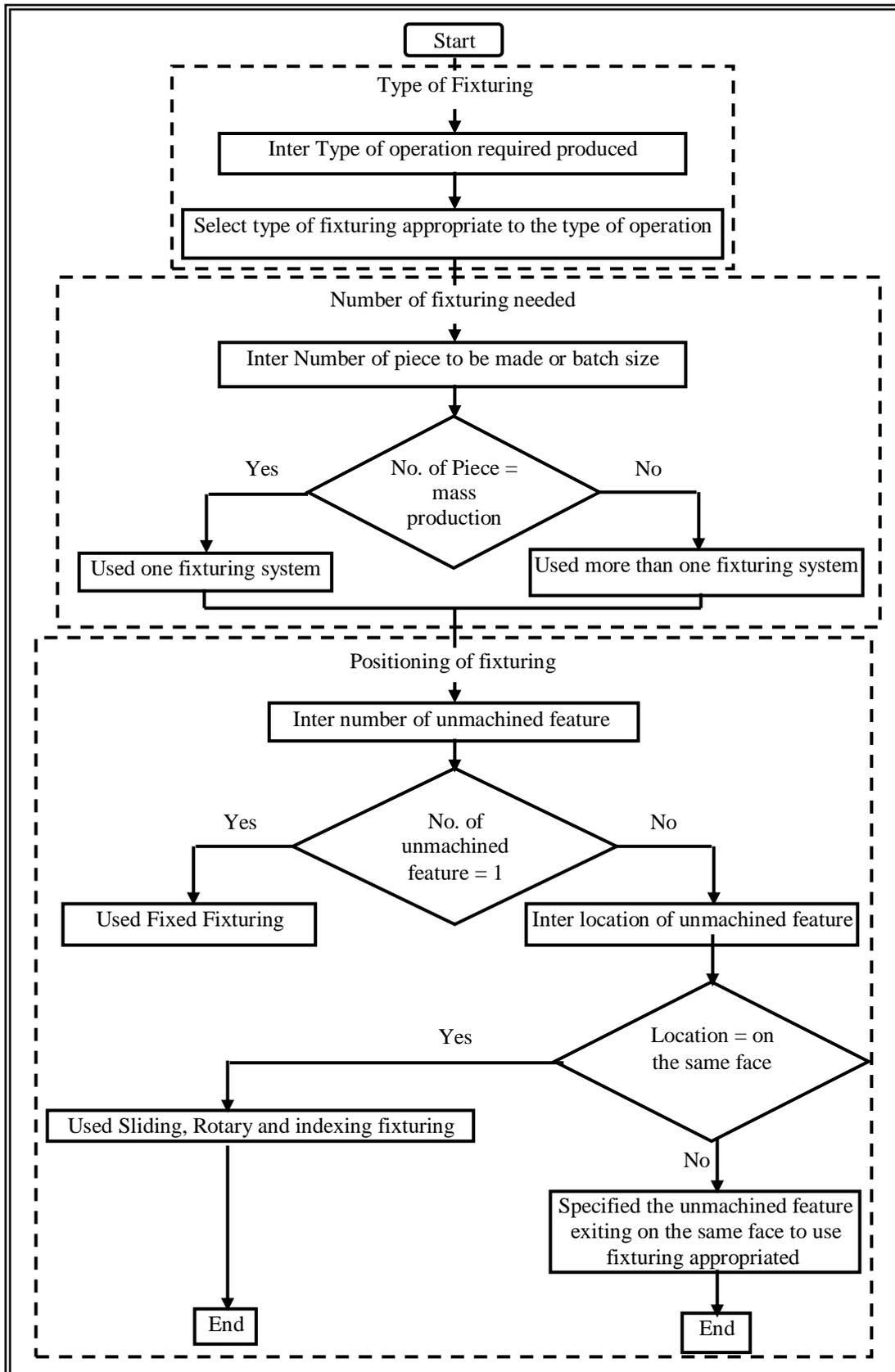
Fig. 5. Algorithm for Fixturing Plan.
