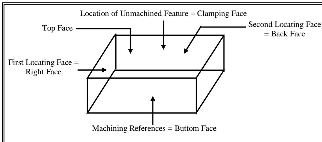
Fig.6. The Rule Used in Constraint Uniform Polyhedra Workpiece.
