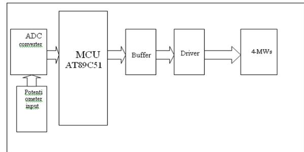
**Fig. 17. Block Diagram of the Control Circuit.**
