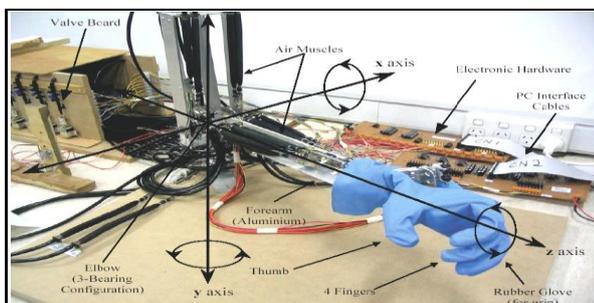
**Fig. 1. The Physical Hand and Arm Comprises 4 Fingers.**
