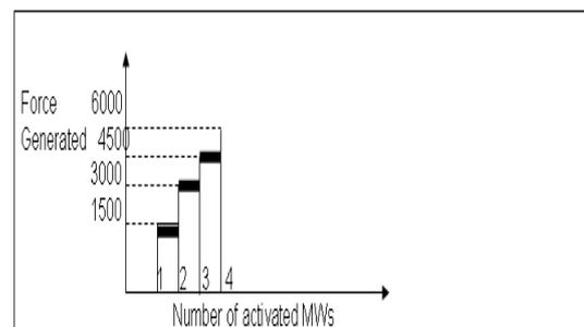
**Fig. 18. Force Generated as a Function of no. of Activated MWs.**
