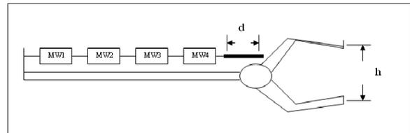
Fig. 12. Schematic of Gripper Controlled by MWs Actuators.
