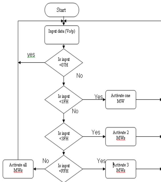
**Fig. 15. The Flow Chart of the Control Program.**
