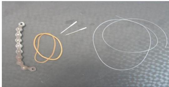
Fig. 5. The Components of a Single Finger.
