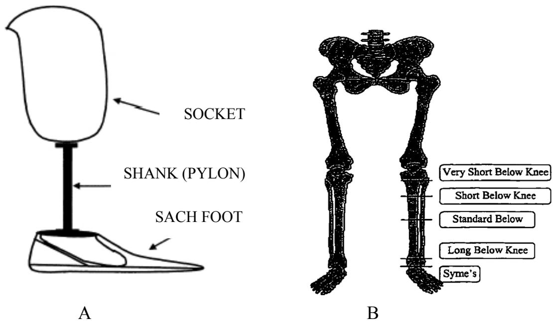
FIGURE ( 1 ) A-COMPONENT OF PROSTHETIC BK, B -PROSTHESES LEVELS
