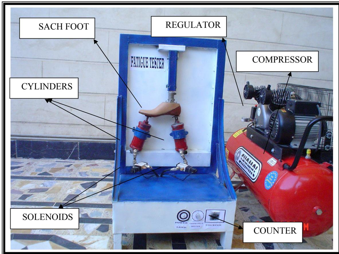
FIGURE( 3 ) FATIGUE FOOT TESTER
