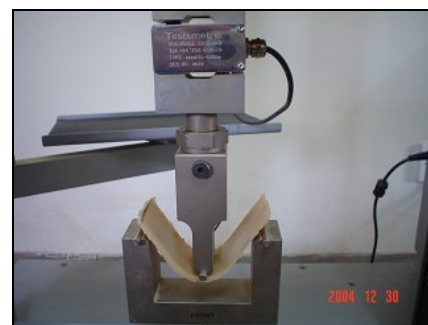
Fig.4 Bending test of socket
