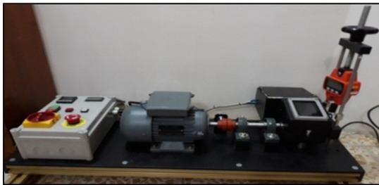
Fig. 3. Fatigue and creep- fatigue interaction test machine.
