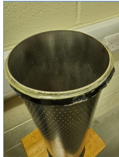
Fig. 1. Illustrates the layout of a single-layer perforated liner pattern utilized at this work.
