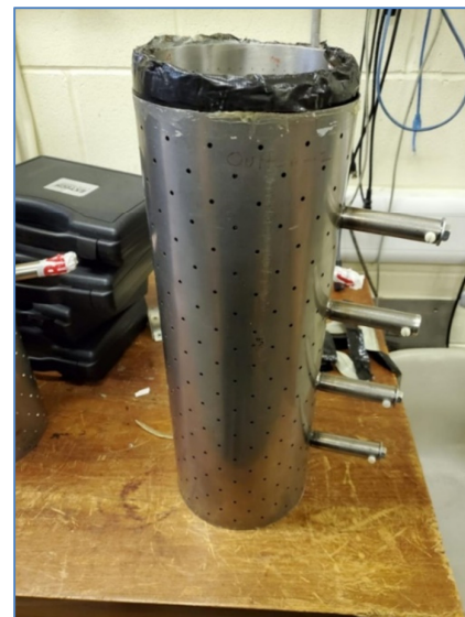
Fig. 2. Illustrates the layout of a double-layers perforated liner pattern utilized at this work.
