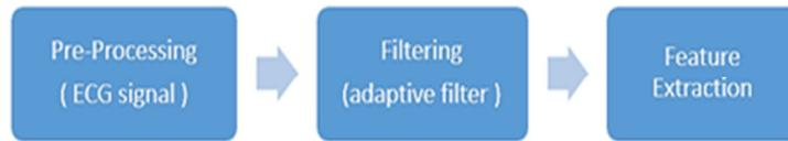
Fig. 5. ECG signal-processing stages.
