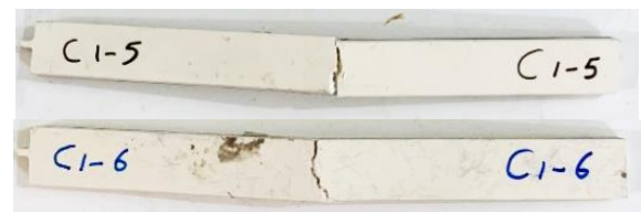
Fig. 12. Samples tested in flexural
