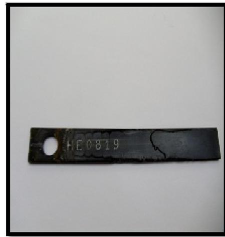
Fig. 8. Protective Layer on Carbon Steel Specimen.
