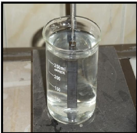
**Fig.1. Carbon Steel Specimen Immersed In Mixture of Sodium Phosphate And Sodium Gluconate.**
