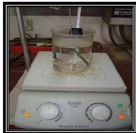
**Fig. 2. Carbon Steel Specimen Immersed in Mixture of Corrosion Inhibitor on Hot Plate and Stirrer at Medium Velocity .**
