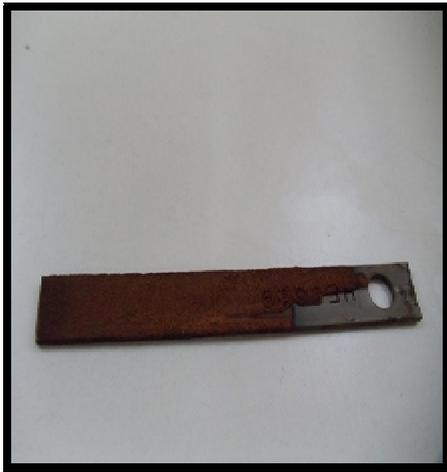
Fig. 7. Uniform Corrosion on Carbon Steel Specimen.
