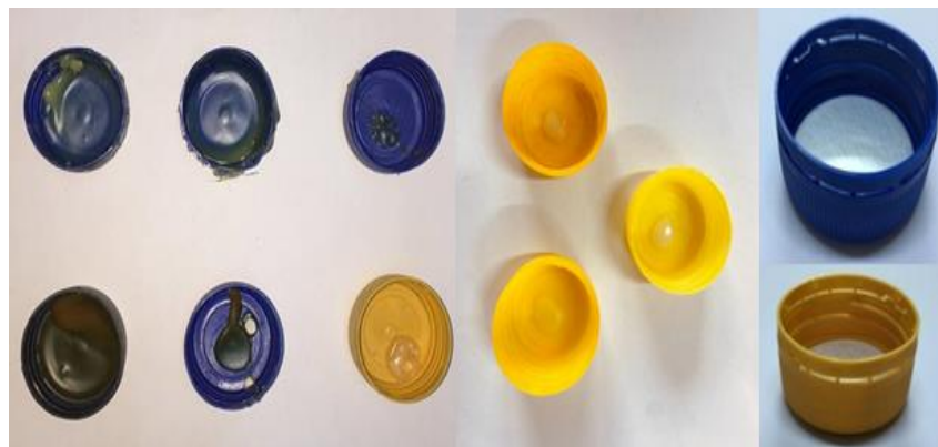
Fig. 6. Glued and glued-sealed caps: (a) glued cap by C.C.S machine (b) glued caps by N.C.S machine (c) cap sealed by the developed machine
