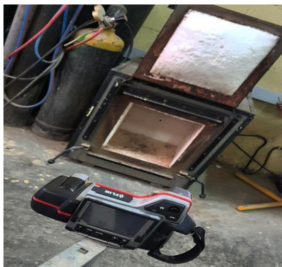
Fig. 3. Capturing thermal image of 3D printer heater
