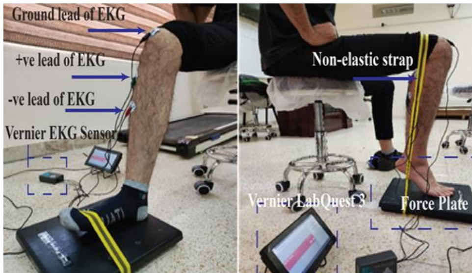
Fig. 1. The experimental setup. The positive and negative electrodes were placed on the upper part of the dominant leg's Tibialis Anterior muscle for each participant. Additionally, the positive and negative electrodes were positioned on the lateral side of each subject's gastrocnemius muscle A-The dorsiflexion setup. B-The plantarflexion setup.
