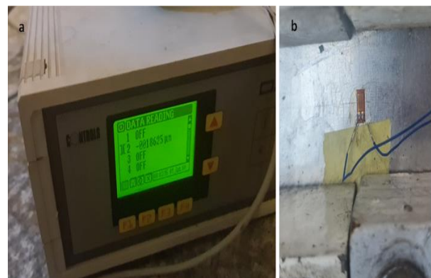
Fig. 6: a) Strain meter device; b) Strain gauge paste on the specimen.
