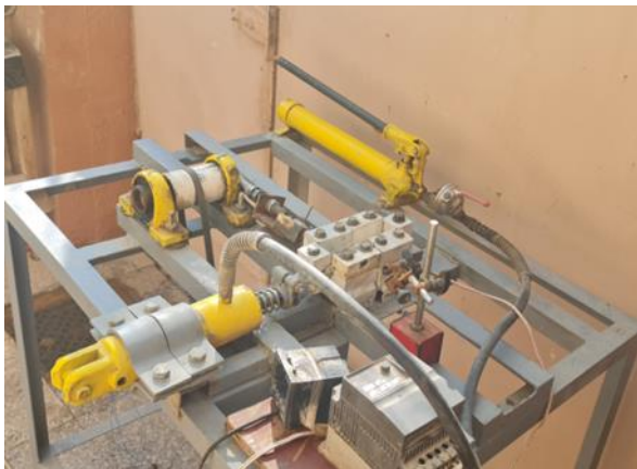
Fig. 8. Section of the fatigue device
