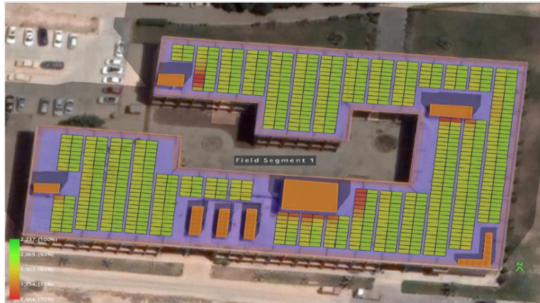
Fig. 3. Implementation of rooftop solar panels and assesment of their susceptibility to shading through HeliScope software
