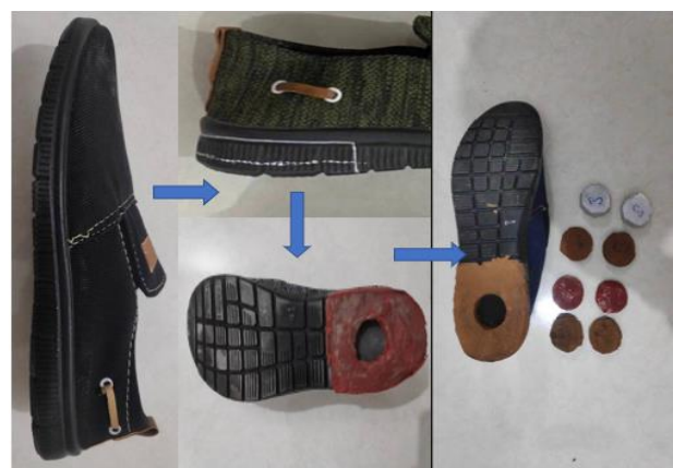
Fig. 1. Preparation of shoes. Starting from cutting the entire heel area and re-casting it with the used materials, according to the dimensions and areas given by the program.
