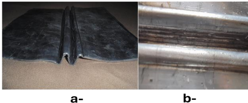
Fig. 18. Formed lead sheet (a) and penetrating lines on surface (b)
