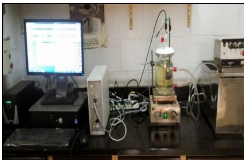
Fig. 1. Complete system set-up for polarisation measurements
