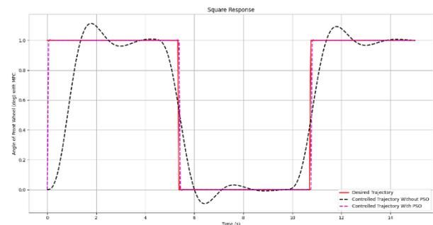
Fig. 10. Square response for the angle of the front tire  $\delta_f$
