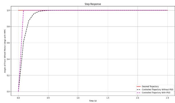
Fig. 7. Step response for the angle of the front wheel motor  $\theta_{m2}$
