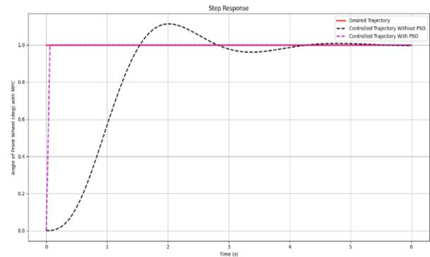
Fig. 8. Step response for the angle of the front tire  $\delta_f$
