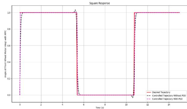
Fig. 9. Square response for the angle of the front wheel motor  $\theta_{m2}$
