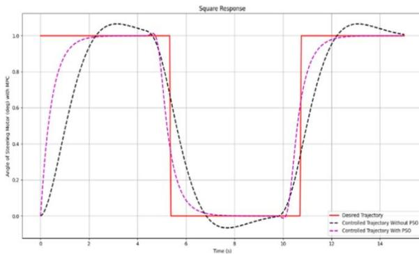
Fig. 6. Square response for the angle of a steering motor  $\theta_{m1}$
