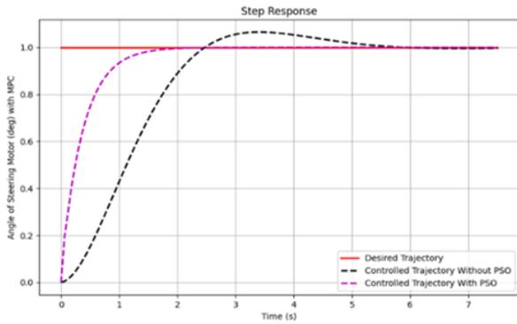
Fig. 5. Step response for the angle of a steering motor  $\theta_{m1}$
