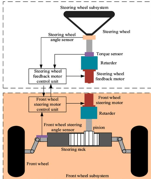
Fig. 1. Steering-by-wire System [2]
