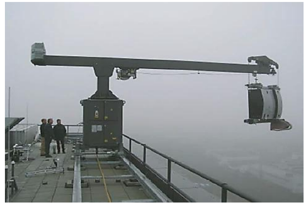
Fig. 15. Facade cleaning robot for a high-rise building in Munich, Germany [63]
