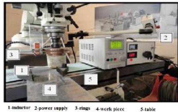
**Fig. 1. Photograph of magnetic abrasive machine supply.**
